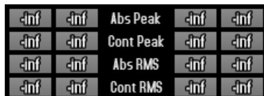
Absolute Peak is the highest amplitude in the signal since playback was started, and Continuous Peak is the highest amplitude in the current frame. Absolute Peak can be set in the preferences to reset every time host play is pressed, or to remain until one of the readouts is clicked.
