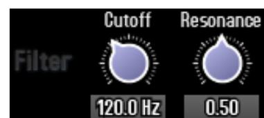
The filter is applied to both the source and reference inputs, and the filtered signal is sent to the oscilloscope, spectral displays, volume meters and dynamics meters.
